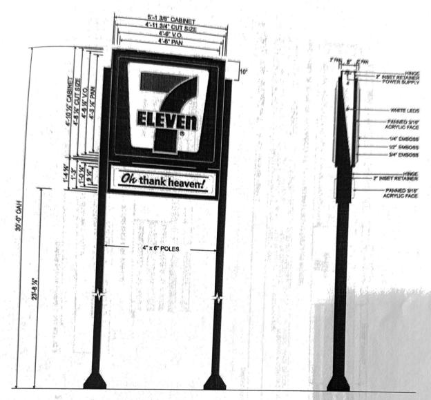
MANUFACTURE & SHIP TWO (2) M25 D/F INTERNALLY ILLUMINATED "MAIN ID" SIGN CABINETS.
